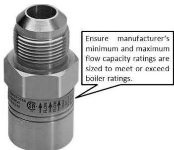
Figure 70 - Excess Flow Valve (EFV)
